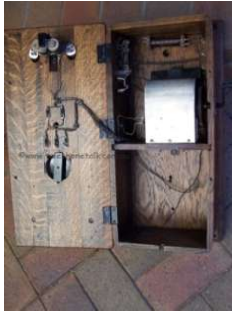
The 135 MW (Magneto Wall) - Manufactured by British Ericsson in the UK. Note the earlier type 35MW had the Solid Back Transmitter, whereas this type 135 used an Inset Transmitter.
