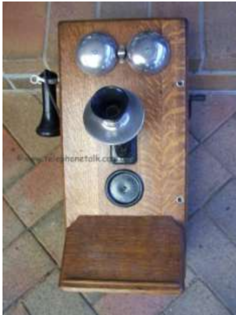
The 135 MW (Magneto Wall) - Manufactured by British Ericsson in the UK. Note the earlier type 35MW had the Solid Back Transmitter, whereas this type 135 used an Inset Transmitter.
