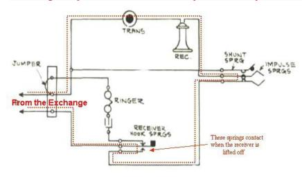
Following the red (dotted) lines added to the circuit diagram, we could see that the transmission currents from and to the telephone exchange would pass through the transmitter (TRANS) and receiver (REC) in series.
