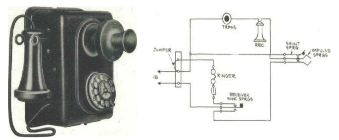
Although the circuit is electrically the same, we will deal with the circuit principles by looking at the circuit diagram for the Metal version of the Automatic Electric Co telephone, purely because it is drawn in a manner that is easier to understand. Immediately obvious in this preceding circuit is the lack of an Induction Coil. This is often called and Anti Side-Tone Induction Coil, or ASTIC.
